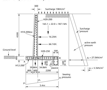
Therefore the horizontal force on 1 m length of wall is given by:
