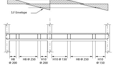
**Figure 7.18**Typical arrangement of shear reinforcement
