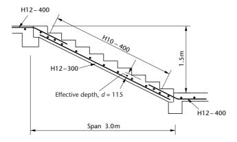
Try a 140 mm thick waist, effective depth, d = 115 mm. This would give an initial estimate of the span-effective depth ratio of 26.1 (3000/115) which, from table 6.10, lies a little above the basic value for a 'lightly stressed' simply supported slab.
