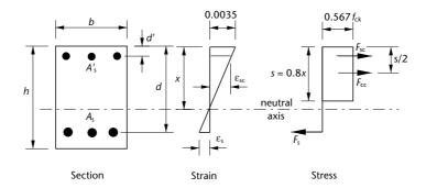
The basic equations derived for a rectangular section as shown in figure 9.7 and with a rectangular stress block are:
