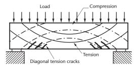
Figure 5.1 Principal stresses in a beam
