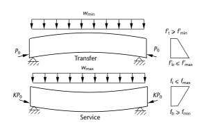
Figure 11.10 Prestressed beam at transfer and service
