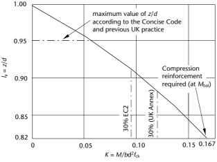
The percentage values on the K axis mark the limits for singly reinforced section with moment redistribution applied (see section 4.7 and table 4.2)
