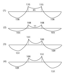
**Figure 3.6**Bending-moment diagrams (kN m)
