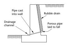
**Figure 10.29** Drainage layer
