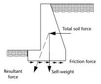
Bending, shear, and deflections of such walls are usually insignificant in view of the large effective depth of the section. Distribution steel to control thermal cracking is necessary, however, and great care must be taken to reduce hydration temperatures by mix design, construction procedures and curing techniques.
