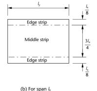
**Figure 8.8**Division of slab into middle and edge strips
