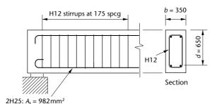
Total ultimate load on beam  $= 200 \times 8.0 = 1600 \, \text{kN}$  Support reaction  $= 1600/2 = 800 \, \text{kN}$  Shear,  $V_{\text{Ef}}$  at face of support  $= 800 - 200 \times 0.3/2 = 770 \, \text{kN}$  Shear,  $V_{\text{Ed}}$  distance d from face of support  $= 770 - 200 \times 0.65 = 640 \, \text{kN}$
