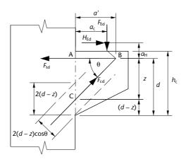
**Figure 7.22**Strut and tie system in a corbel
