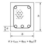
**Figure 6.1** Definition of axis distance, *a*
