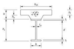
Figure 13.7 Composite section dimensions
