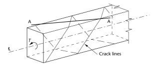
**Figure 5.15**Torsional reinforcement
