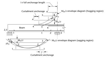
$\Delta F_{\rm td}$  is a maximum where the shear force is a maximum at sections of zero moment, and  $\Delta F_{\rm td}$  is zero at the maximum moment near to mid-span and the interior support.
