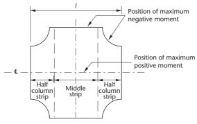
Width of half column strip = I/4 with no drops or = half drop width when drops are used
