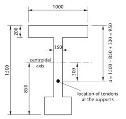
Figure 11.27 Shear reinforcement example
