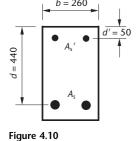
Design example with compression reinforcement,
