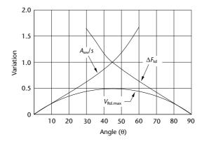
**Figure 5.3** Variation of  $V_{\rm Rd,\,max}$ ,  $\Delta F_{\rm td}$  and  $A_{\rm sw}/s$
