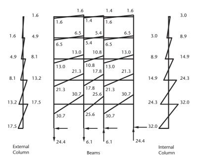
Figure 3.21 Moments (kNm) and reactions (kN)
