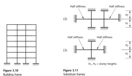
When considering the critical loading arrangements for a column, it is sometimes necessary to include the case of maximum moment and minimum possible axial load, in order to investigate the possibility of tension failure caused by the bending.
