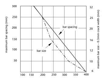
Stress in reinforcement under quasi-permanent load (N/mm²) (see sections 6.1.3 and 6.1.7)
