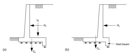
Figure 10.26 Cantilever walls
