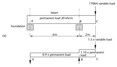
**Figure 2.3**Uplift calculation example
