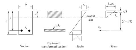
Cracked section – strain and stress distribution
