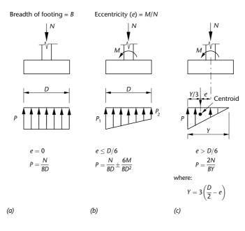
**Figure 10.3**Pad-footing – pressure distributions
