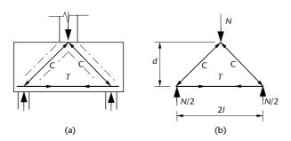
From the geometry of the force diagram in figure 10.20b:
