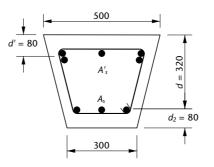
**Figure 9.17**Non-rectangular section example
