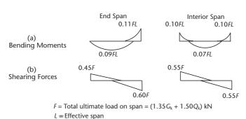
The possibility of hogging moments in any of the spans should not be ignored, even if it is not indicated by these coefficients. For example, a beam of three equal spans may have a hogging moment in the centre span if  $Q_k$  exceeds  $0.45G_k$ .
