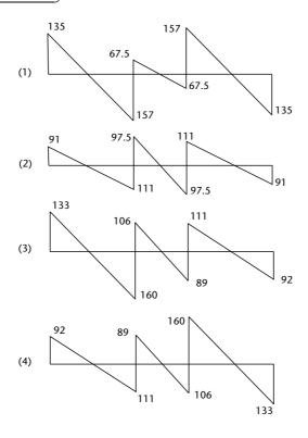
**Figure 3.15**Bending-moment and shearing-force envelopes
