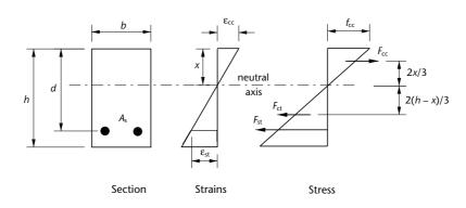
**Figure 4.31**Triangular stress block – uncracked section
