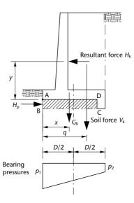
**Figure 10.28** Forces on a cantilever wall
