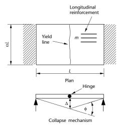
Internal energy absorbed by rotation along the yield line is moment  $\times$  rotation  $\times$  length  $= m\phi\alpha L$
