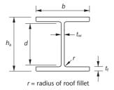
For class 1 and class 2 I-beams with a predominately uniformly distributed load the design shear stresses are seldom excessive and the shear area,  $A_{\rm v}$  may be conservatively taken as the web area so that
