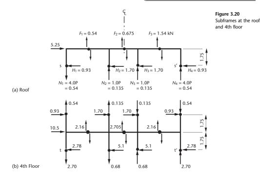
By inspection, there is tension in the two columns to the left and compression in the columns to the right; and by assumption 2 the axial forces in columns are proportional to their distances from the centre line of the frame. Thus
