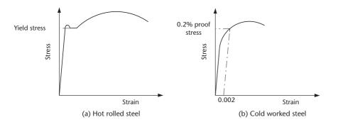
**Figure 1.7**Stress–strain curves for high yield reinforcing steel
