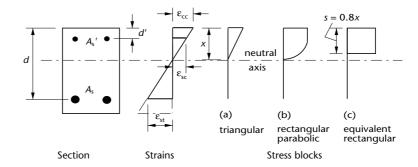
Figure 4.3 shows the cross-section of a member subjected to bending, and the resultant strain diagram, together with three different types of stress distribution in the concrete:
