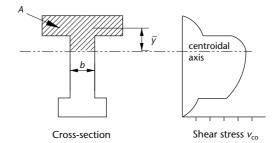
**Figure 11.26**Shear stress distribution
