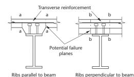
**Figure 13.14**Transverse reinforcement in the concrete flanges
