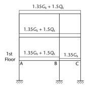
(a) Critical loading arrangement for centre columns at 1st floor
