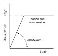
Figure 4.2 Short-term design stress–strain curve for reinforcement
