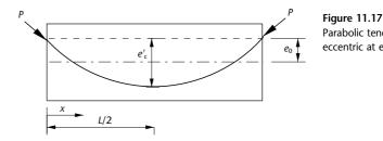
If the prestress force does not lie at the centroid of the section at the ends of the beam, but at an eccentricity  $e_0$  as shown in figure 11.17, the expression for deflection must be modified. It can be shown that the deflection is the same as that caused by a force P acting at a constant eccentricity  $e_0$  throughout the length of the member, plus a force P following a parabolic profile with mid-span eccentricity  $e'_{c}$  as shown in figure 11.17.
