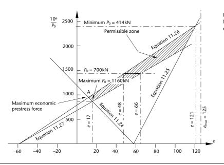
**Figure 11.13** Magnel diagram for example 11.5
