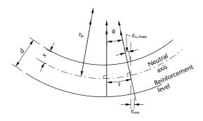
The strains in the concrete and tensile reinforcement depend on the areas of reinforcement provided and their stresses. Thus for a particular member section and a pattern of loading, it is possible to determine a span-effective depth ratio to satisfy a particular a/L or deflection/span limitation.
