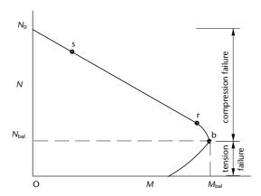
At point b on the interaction diagram of figure 4.20,  $N = N_{\text{bal}}$ ,  $M = M_{\text{bal}}$  and  $f_{\text{s}} = -0.87 f_{\text{yk}}$ . When the design load  $N > N_{\text{bal}}$  the section will fail in compression, while if  $N < N_{\text{bal}}$  there will be an initial tensile failure, with yielding of reinforcement  $A_{\text{s}}$ .
