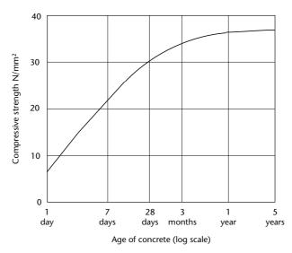
design load. European Codes, however, do not permit the use of strengths greater than the 28-day value in calculations, but the modulus of elasticity may be modified to account for age as shown later.
