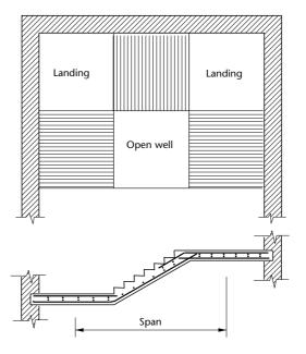
**Figure 8.19**Stairs spanning into landings
