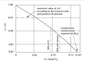
**Figure 4.5** Lever-arm curve
