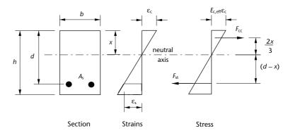
For a given moment, M, and from elastic bending theory, the curvature of the section,  $(1/r)_{\rm uc}$ , is given by
