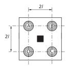
**Figure 10.21** Four-pile cap
