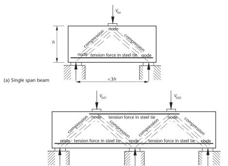
**Figure 7.25** Truss and tie models
