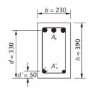
**Figure 7.8**Beam doubly reinforced to resist a hogging moment
