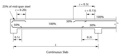
The effective span of the slab may be taken as the clear distance between the face of the supports plus a distance at both ends taken as the lesser of (a) the distance from the face of the support to its centreline and (b) one-half of the overall depth of the slab.
