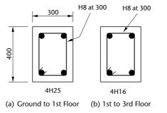
Note: the link spacing is reduced to 0.60 x these values for 400mm above and below each floor level and at laps below 1st floor level
