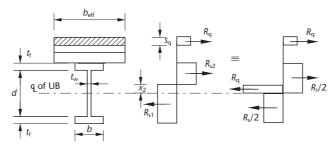
(b) Neutral axis in the steel web  $x > h + t_f : R_c < R_w$
