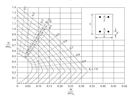
These equations are not suitable for direct solution and the design of a column with symmetrical reinforcement in each face is best carried out using design charts as illustrated in figure 9.8. Sets of these charts can be found in the Concise Eurocode (ref. 24), the Manual for the Design of Concrete Structures (ref. 29) and the website www.eurocode2.info.
