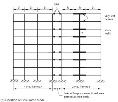
whereas this would normally be of a secondary magnitude. To overcome this the cross-sectional areas of all the beams in the model may be increased say to  $1000 \,\mathrm{m}^2$  and this will virtually remove the effects of axial shortening in the beams.
