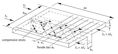
**Figure 5.6**Shear between flange and web
