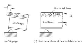
**Figure 13.10**Slippage and horizontal shear
