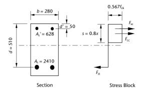
**Figure 4.11**Analysis example, doubly reinforced section
