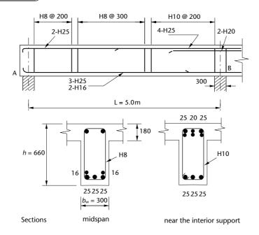
Calculating  $M/(b_{\rm f}d^2f_{\rm ck})$  and using the lever-arm curve, it is found that  $l_{\rm a}=0.95$
