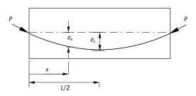
Parabolic tendon profile eccentric at ends of beam
