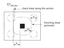
**Figure 10.22** Critical sections for shear checks
