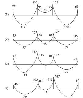
**Figure 3.13**Beam bending-moment diagrams (kNm)
