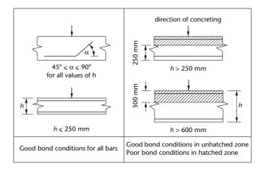
Good bond conditions are considered to be when (a) bars are inclined at an angle of between  $45^{\circ}$  and  $90^{\circ}$  to the horizontal or (b) zero to  $45^{\circ}$  provided that in this second case additional requirements are met. These additional conditions are that bars are
