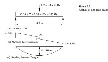
Figure 3.3 shows the values of ultimate load required in the calculations of the shearing forces and bending moments.
