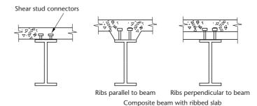
Figure 13.2 Composite floor beams
