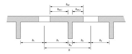
So that for the interior span of a symmetrical T-beam with  $b_1 = b_2 = b'$  and  $l_0 = 0.7l$
