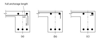
Precast concrete construction, however, presents a more serious problem since the requirements of tie forces and simple easily constructed joints are not always compatible. Unless the required tie forces can be provided with the bars anchored by hooks and bends in the case of column and wall ties, an analysis of the structure must be performed to assess the remaining stability after a specified degree of structural damage.
