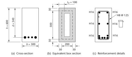
The beam cross-section is shown in figure 7.30(a). The steps in the calculations are numbered as outlined in the previous description of the design procedure. The characteristic strengths of the concrete and steel are  $f_{\rm ck}=30\,{\rm N/mm^2}$  and  $f_{\rm yk}=500\,{\rm N/mm^2}$ .
