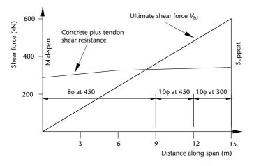
at 300 mm centres in the outer 3 metres  $(A_{\rm sw}/s=0.523)$  changing to 10 mm links at 450 mm centres  $(A_{\rm sw}/s=0.349)$  between 3 and 6 m from the end of the beam and then 8 mm at 450 centres  $(A_{\rm sw}/s=0.223)$  throughout the rest of the span as shown in figure 11.28.
