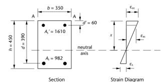
Figure 4.21 Non-symmetrical section *M*–*N* interaction example
