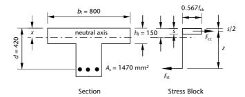
**Figure 4.13** Analysis example of a T-section,  $s < h_f$
