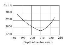
**Figure 9.14**Design chart for unsymmetrical column example
