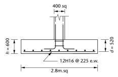
Assume a footing weight of 150 kN so that the total permanent load is 1150 kN and base the design on the *Prescriptive Method*.
