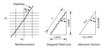
If the ultimate moments of resistance provided by main and transverse steel are  $m_1$  and  $m_2$  per unit width, it follows that for equilibrium of the vectors shown, the ultimate moment of resistance normal to the yield line  $m_n$  per unit length is given by
