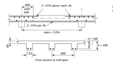
Figure 8.16 Ribbed slab
