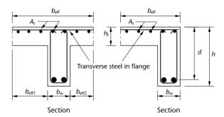
**Figure 7.10** T-beam and L-beam
