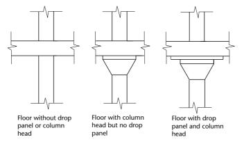
Figure 8.10 Drop panels and column heads
