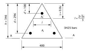
**Figure 4.23** Non-rectangular *M–N* interaction example
