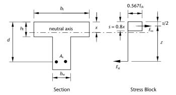
If s is less than the flange thickness ( $h_f$ ), the stress block does lie within the flange as assumed and the area of reinforcement is given by
