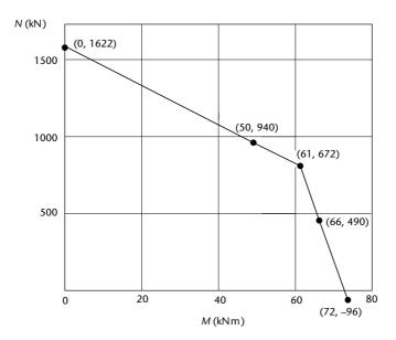
Table 4.4 has been calculated using the fundamental equations with the values of *x* shown. The interaction diagram is shown constructed in figure 4.24.
