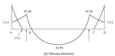
The slab will also carry a direct tension force of
