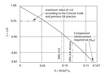
**Figure A.3** Lever-arm curve
