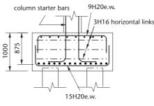
**Figure 10.23**Pile-cap design example
