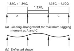
Figure 3.1 Three-span beam
