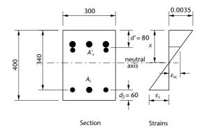
3. From the stress–strain curve and the relevant equations of section 4.1.2 yield strain,  $\varepsilon_y = 0.00217$  for grade 500 steel
