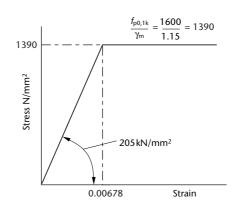
Figure 11.23 Stress–strain curve for prestressing wire
