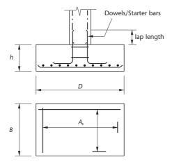
Maximum shear 2.0dPunching shear basic control perimeter = column perimeter +  $4\pi d$ Shear
