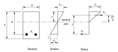
**Figure 4.27**Triangular stress block – cracked section
