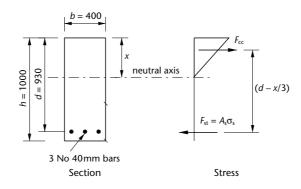
**Figure 6.13**Crack width calculation example
