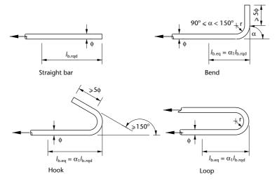
Minimum internal radius of a hook, bend or loop =  $2\phi$  or  $3.5\phi$  for  $\phi \geqslant 16$  mm
