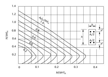
The direct solution of equations 4.37 and 4.38 for the design of column reinforcement would be very tedious and, therefore, a set of design charts for the usual case of symmetrical sections is available in publications such as *The Designers Guide* (ref. 23). Examples showing the design of column steel are given in chapter 9.
