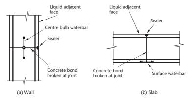
**Figure 12.3** Partial contraction joint
