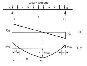
Using the sign convention of figure 3.4 and taking moments about support B:
