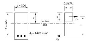
For equilibrium of the compressive and tensile forces on the section
