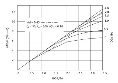
**Figure 4.9**Typical design chart for doubly reinforced beams
