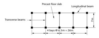
Figure 6.17 Structure layout
