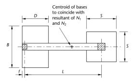
Figure 10.11 Strap footing with shearing force and bending moments for the strap beam
